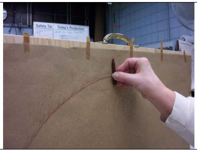
2. Being careful not to press against the template paper while tracing, draw an exact outline of the window opening. Pressing on the template paper may distort the paper and cause the wrong size to be made.
