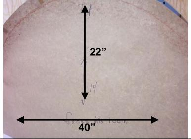
4. Mark the dimensions on the template. Check that the template dimensions match your measurements of the actual window opening.
