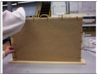
1. Tape acceptable paper over the window opening allowing plenty of overlap.
