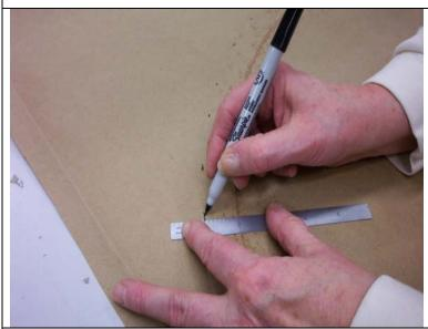
3. Remove the paper from the window opening. If the shade is an outside mount, add the desired amount of overlap to the window outline and draw a second outline around it to match the shape of the finished shade. Be sure to erase the inside line.
